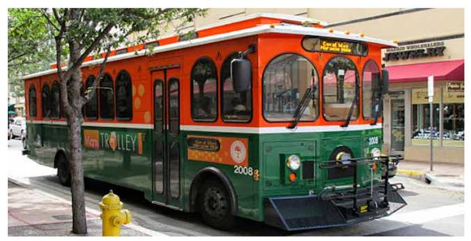
Figure 69: Most trolleys are high floor and low capacity, limiting their usefulness for high ridership service
