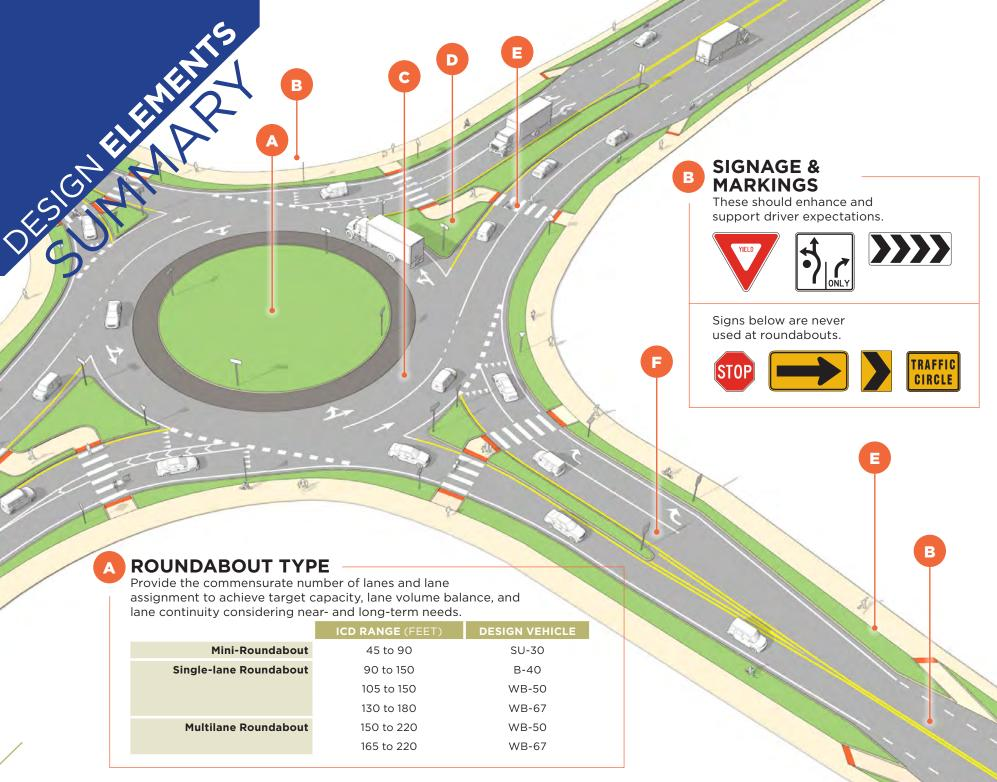
MASSDOT GUIDELINES FOR THE PLANNING AND DESIGN OF ROUNDABOUTS
